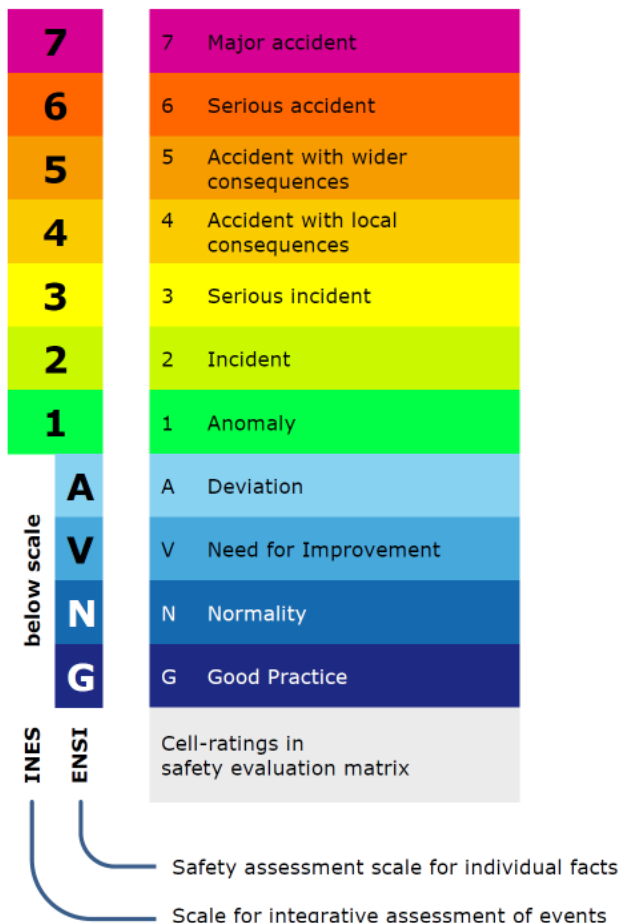
Figure 4: ENSI’s safety assessment scale for individual facts and the International Nuclear and Radiological Event Scale (INES) for the integrated assessment of events
