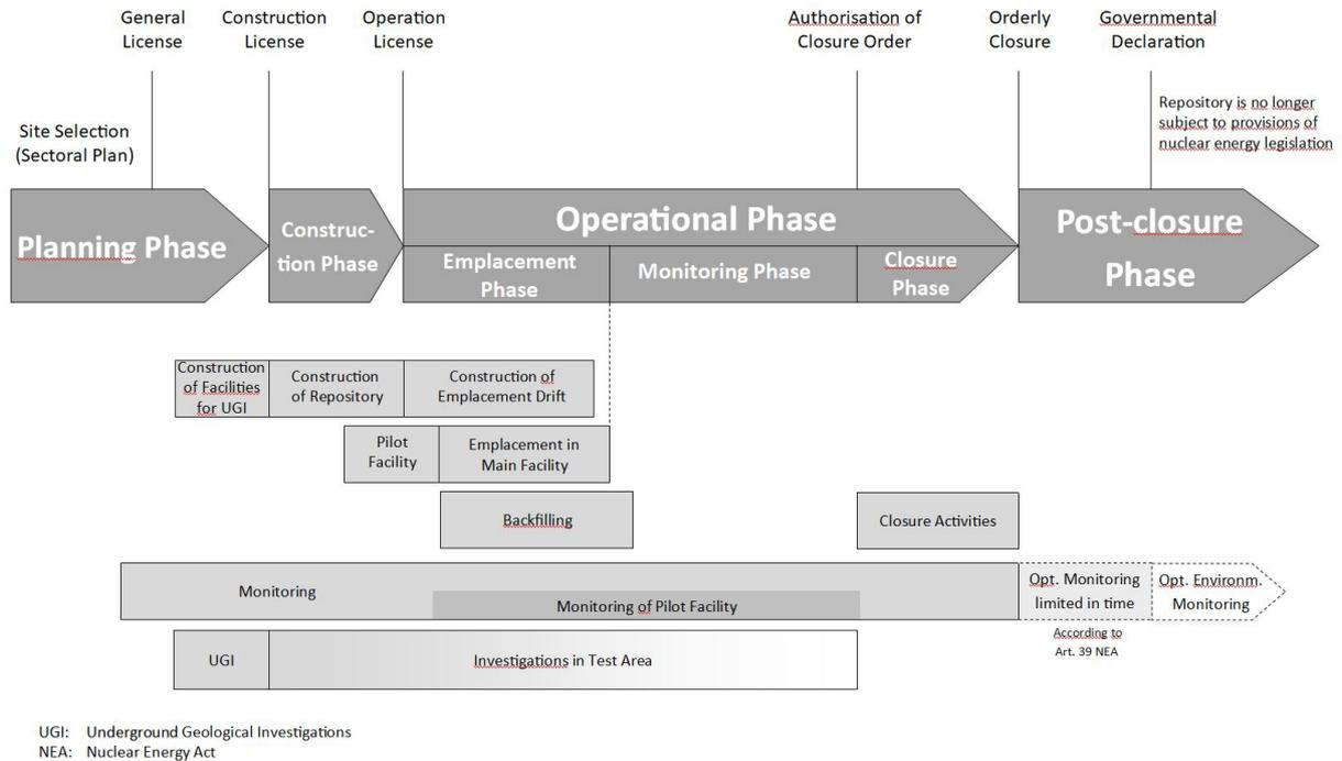
The operational phase of a deep geological repository comprises waste emplacement, the monitoring phase and closure.
