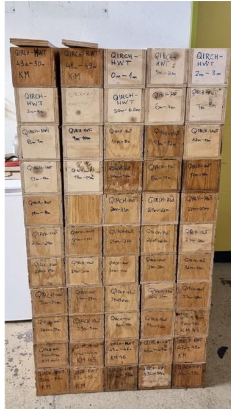
**Figure 4:** Photograph of the Hochwacht drill site (left) and the boxes containing the 1m drill cores from the Hochwacht drill site (right).
